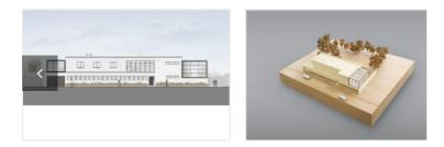
The new extension is designed to be easily removable to allow restoration of the house to its existing condition at some later date, and was prefabricated to minimise disruption to the house and its occupants, and to afford a high degree of control over the quality of finish.
